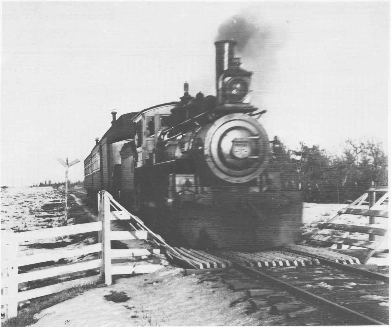
Wisconsin Central No. 52, a 4-4-0 built by Schenectady in 1884, C/n 1896, is pulling a two-car passenger train in this early example of action photography. No. 52 was scrapped in 1905. Courtesy Jerry Lopas collection.
